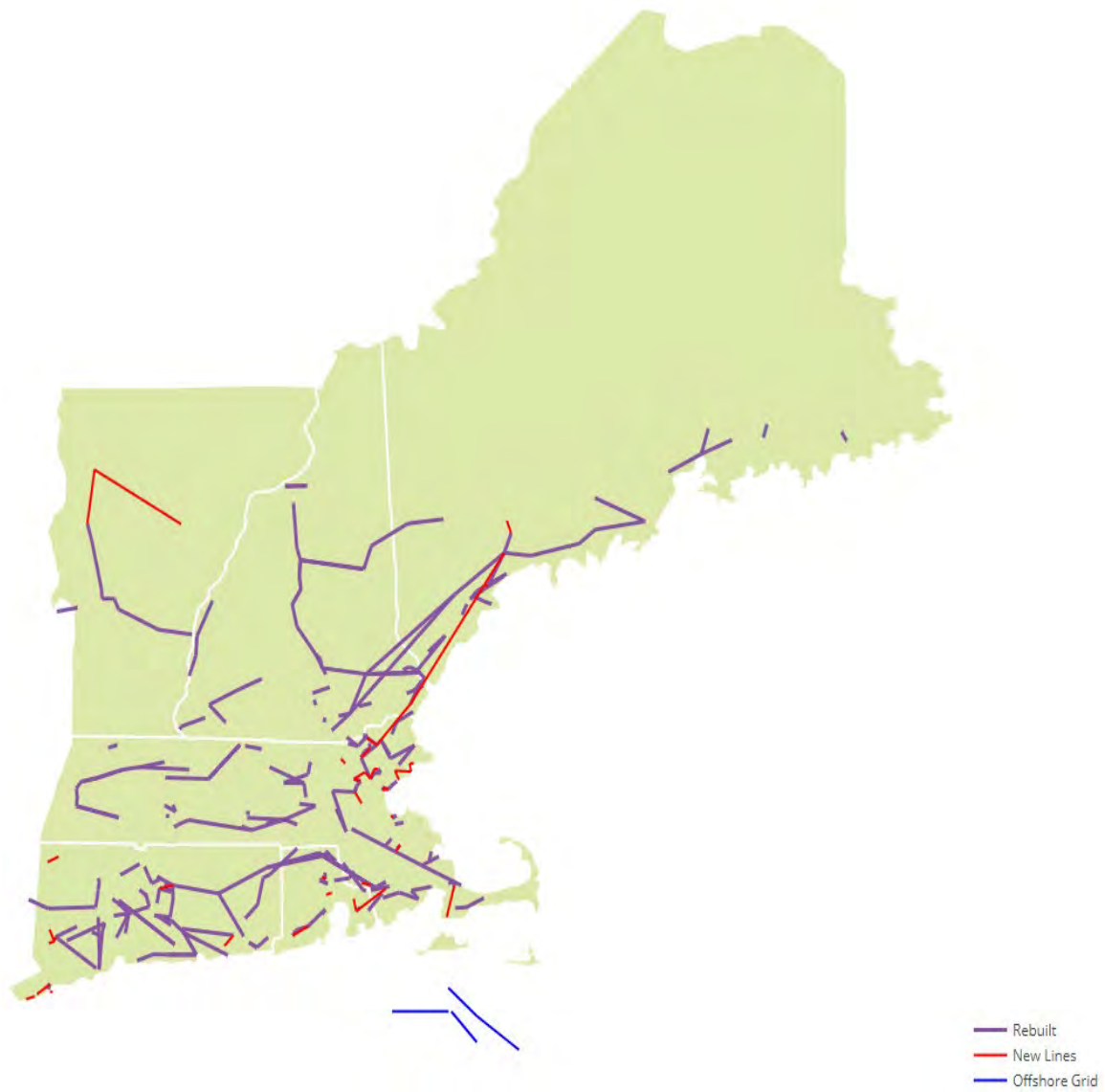
Figure 4-13: Transmission Upgrades and Additions for the New Haven - Essex Roadmap and the Offshore Grid Roadmap
