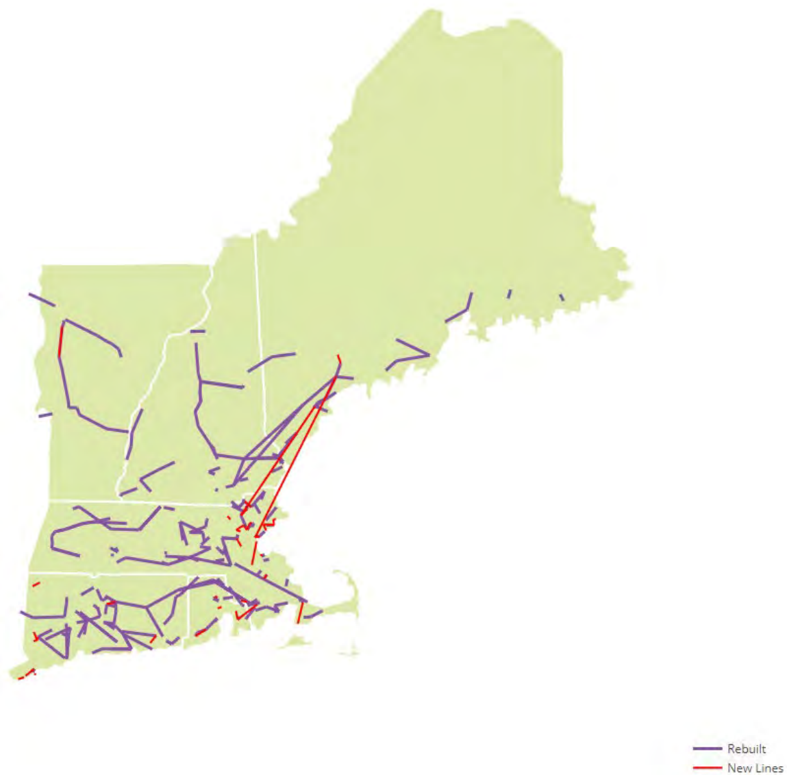
Figure 4-12: Transmission Upgrades and Additions for the PV-20 Roadmap and the DC Roadmap
