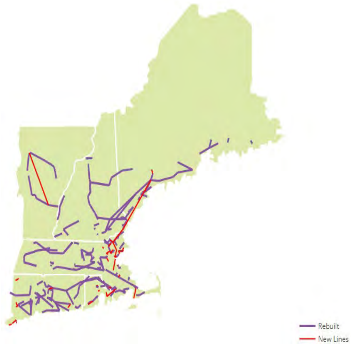
Figure 4-10: Transmission Upgrades and Additions for the Coolidge -Essex Roadmap and the AC Roadmap
